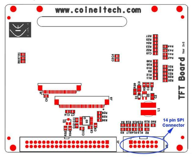
**Note:** Only 14 pin SPI connector is used for 3.2" TFT Board interface. Other Connectors in the board are not used.
